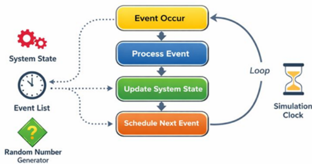
Figure 1 Basic components and event flow of discrete event simulation
