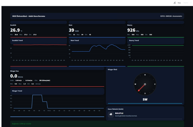
Figure 9 Python-Based User Interface Designed Over Bluetooth Communication.
