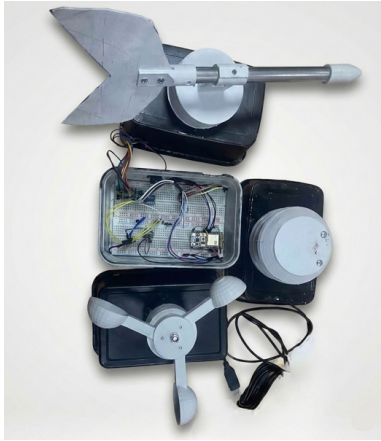
Figure 10 General view of the developed modular meteorological station hardware, including the anemometer, wind vane, and the main control unit.
