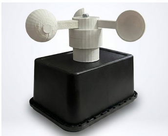
Figure 5 Three-Cup Anemometer Design and Electronic Enclosure Box.
